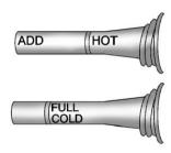
When the engine compartment is hot, the level should be at the HOT mark. When the engine compartment is cool, the level should be at the FULL COLD mark.
